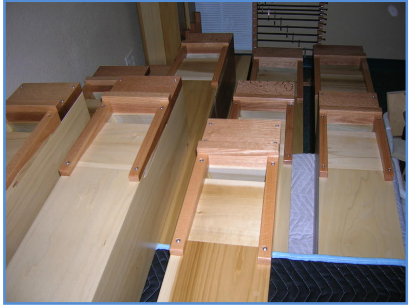
Large wood pipes made of Poplar and Oak laying flat in storage.
