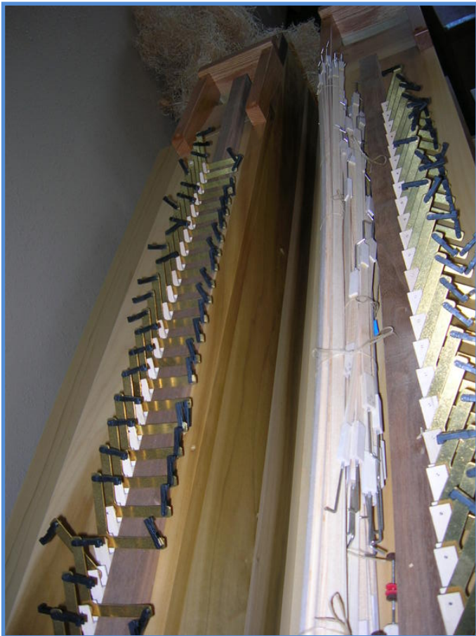
Playing action parts and wood linkages (called trackers).
